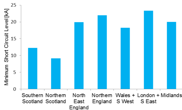
Figure 20 Minimum Short Circuit Level (2014/15)
